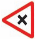
Intersection where the priority is that prescribed by the general priority rule in force in the country
