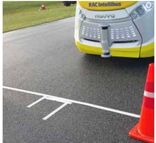
Figure 2: Testing RAC’s Intellibus at RAC’s private track in “Static Object Detection” Test.
